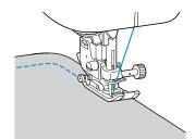
When sewing along a curve while using a zigzag stitch, select a shorter stitch length in order to obtain a finer stitch.
